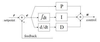
Figure 4. PID controller structure
