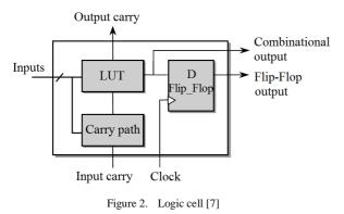
Also, a carry look-ahead data path is included in order to build arithmetic operators and a D-Type Flip-Flop with all its control inputs, allowing registering the output of the logic cell.
