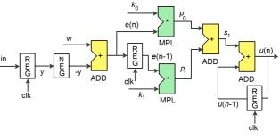
Figure 5. Parallel design of incremental PI algorithm
