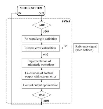
Figure 8. FPGA-based control implementation cycle
