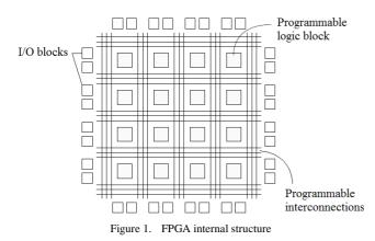
A custom design can be implemented by specifying the function of each logic cell and setting the connection of each programmable switch. The CLBs structures include 2, 4 or more logic cells, also called logic elements. The structure of a logic cell, as the basic grain of the FPGA, is presented in Fig. 2. It consists of a Look-up Table (LUT), which can be configured either as a ROM, RAM or a combinatorial function.
