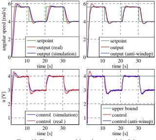
Figure 10. Time responses of the real system and simulation
