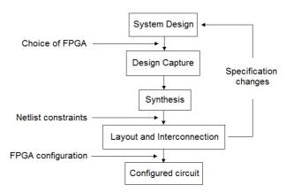
Figure 3. Design process of the circuit
