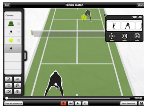
Figure 3. The idAnimate animation tool, with the object selector displayed on the left, the object inspector on the right, the canvas in the center and the animation and playback controls at the bottom.
