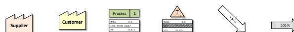
Figure 4. The standard VSM symbols (from left to right): Supplier, Customer, Process, Buffer, External flow, Internal flow.
