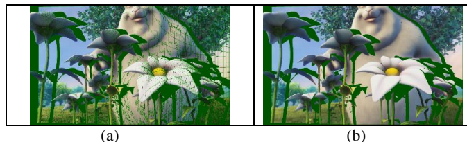
Figure 3: (a) Primary synthesized view with cracks and holes shown in green; (b) cracks are filled by interpolation.
