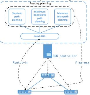
Figure 4. Routing planning example based on TEID
