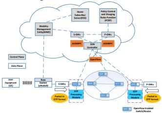
Figure 2. SDN-based mobile core network architecture
