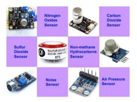
Figure 7. Exemplar Components aboard 3DP Sensors
