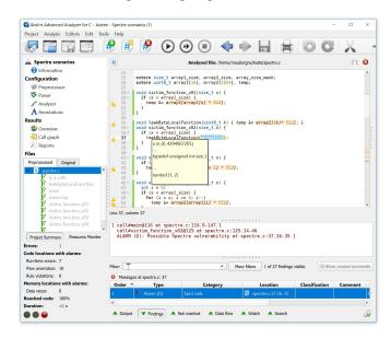
Figure 5. Astrée GUI showing Spectre vulnerability alarm
