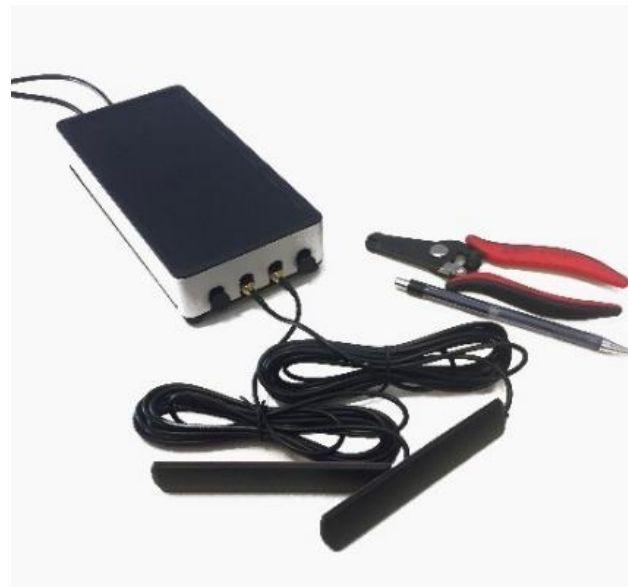
Figure 1. Device under test: a prototype wireless intrusion detection system
