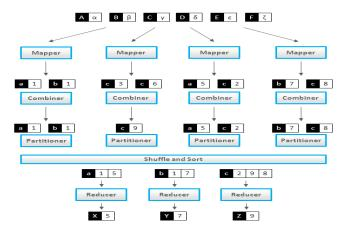
Figure 1b. Map, Shuffle, and Reduce phase example.
