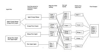
Figure 1a. Map, Shuffle, and Reduce phase example.
