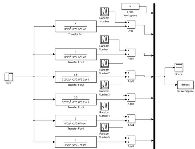
Figure 6. SIMULINK structure for test data generation.
