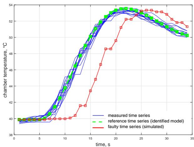
Figure 4. An example for the identified time shift in time series which can be caused by equipment malfunction.
