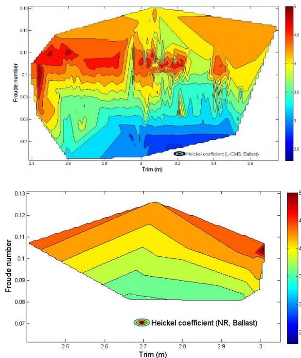
Figure 6. Heickel coefficient distribution vs Froude number and trim for ballast condition. L-CMS (up) and NR (down) data.
