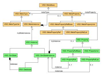
Figure 3. VSD data model (top: metadata, bottom: instance data).
