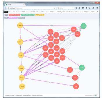
Figure 9. 3D simulation model data (excerpt) of an industrial robot stored within Neo4j.
