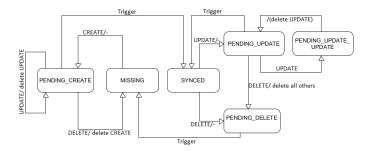
Figure 7. State machine of the change tracking mechanism.
