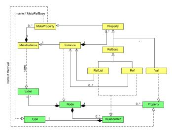
Figure 4. Data mapping of the synchronization component (top: VSD data model, bottom: Neo4j data model).
