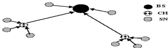
Figure 2. The Network Model for the WEPCS Algorithm.
