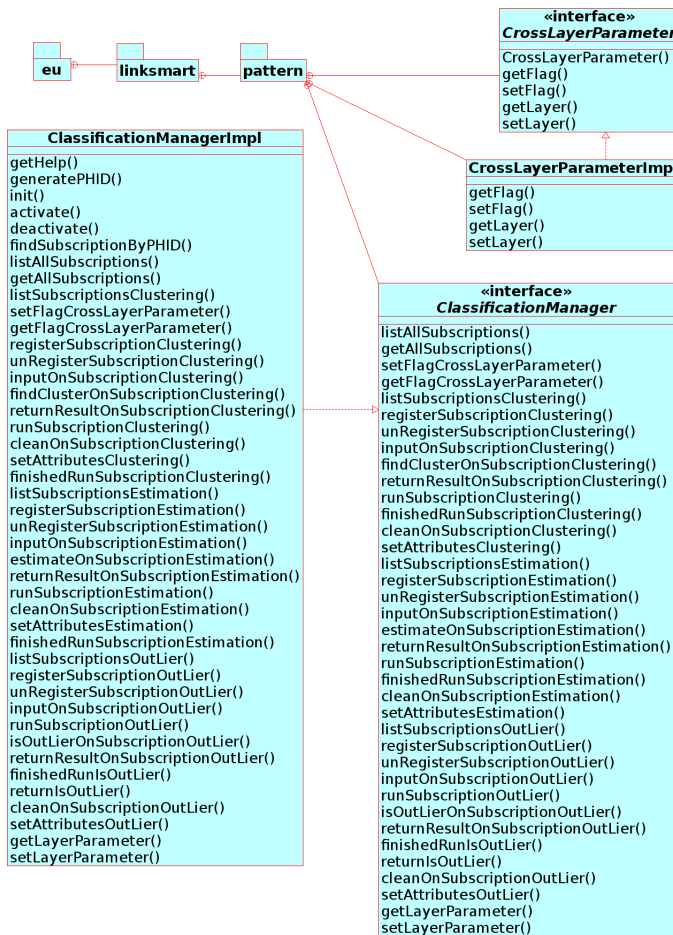
Figure 4. Class diagram of the cross-layer parameters and service implementation in the pattern recognition module.
