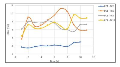
Figure 6. Jitter during multiple caching traffics in the network.
