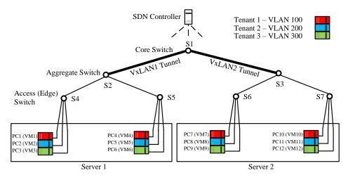
Figure 1. A multi-tenancy architecture used in both 1) VMWare/Mininet and 2) GNS3 tools.
