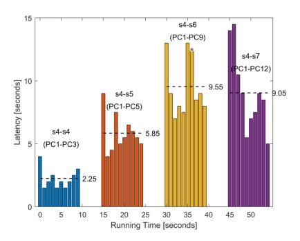
Figure 4. Latency in inter-VLAN communications
