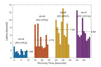
Figure 2. Latency analysis for the intra-VLAN communications
