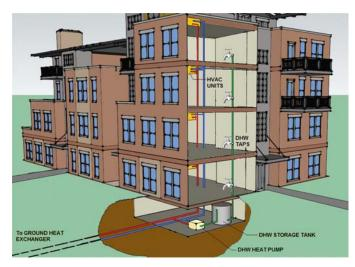
Figure 2. Example of geoexchange system for space conditioning and domestic hot water
