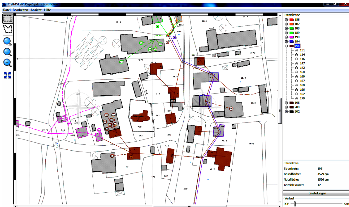
Figure 1. An interactive cadastral map showing boundaries of land parcels and buildings, as well as the structure of an existing power grid.
