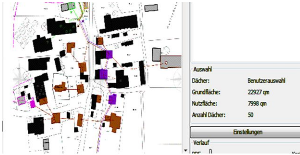
Figure 3. Selection of a group of buildings for estimating available roof surface area for additional PV panel installations.
