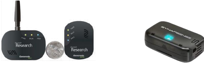
Figure 5. Sensor nodes for data centre monitoring. Left: Genomotes from Microsoft Research; Right: ThermaNode from SynapSense
