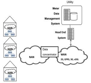
Figure 2. Typical AMI architecture
