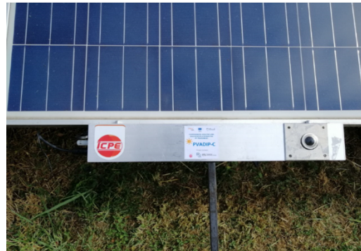
Figure 6. The sensor platform mounted on a solar panel
