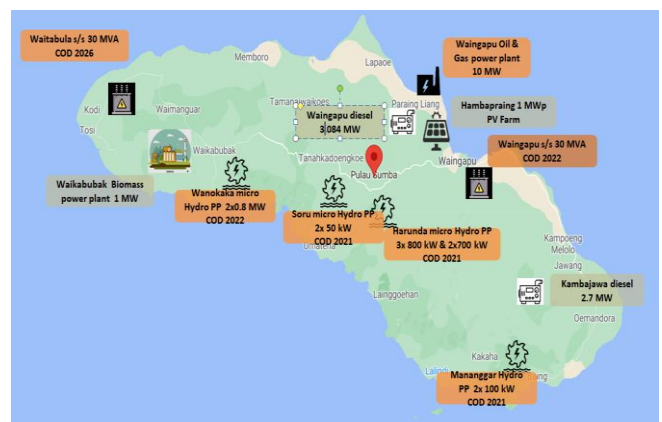
Figure 1. Sumba distribution grid and its planning expansion
