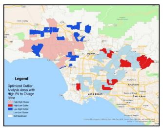
Figure 11. Optimized outlier analysis of EV chargers in areas of Los Angeles with calculated EV-to-charger ratios greater than 18.7.
