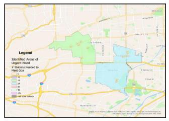
Figure 14. Sample area in Los Angeles County with identified quantity of new EV charging stations needed to meet goal ratio of 18.7.
