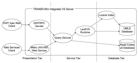
Figure 1. TRANSFoRm VS Server Architecture
