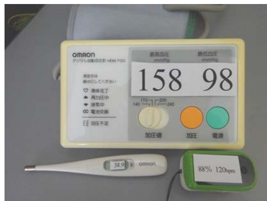
Figure 1. Blood-pressure manometer, thermometer and pulse oximeter, which we put paper on to reproduce an abnormal value.
