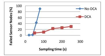
Figure 9. Sampling Time vs Failed rate of 20 intruders
