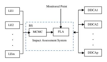
m: the number of sensor nodes that are queried by the BSp: the number of sensor nodes around the monitored point LEi: the location of intruder i
