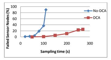
Figure 10. Sampling Time vs Failed rate of 30 intruders
