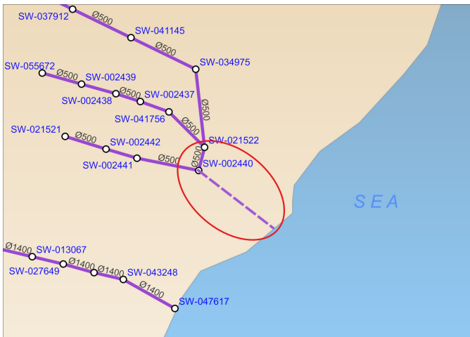
Figure 3. Sample error of the missing discharge line.
