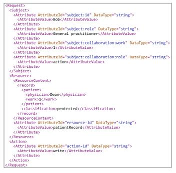
Figure 7. Example of an XACML access request
