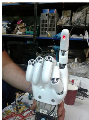
Figure 3. Integrating the Slip Sensor
