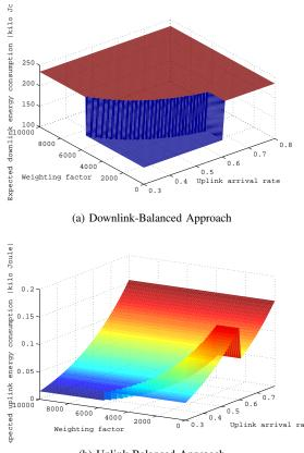
(b) Uplink-Balanced Approach Figure 5. The expected energy consumption versus the arrival rate of uplink users and the weighting factor [45].
