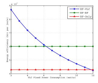
Figure 4. Energy efficiency against the fixed power of the VLC system [44].
