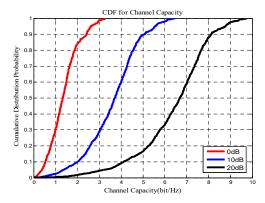
Figure 6. Cumulative Distribution Function for Channel Capacity
