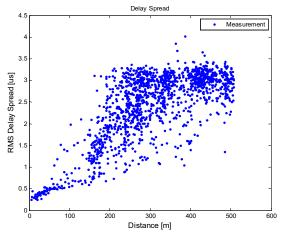
Figure 4. RMS Delay Spread according to the distance
