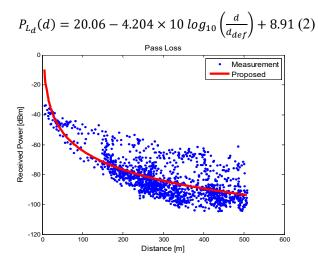
Figure 3. Path loss according to the distance
