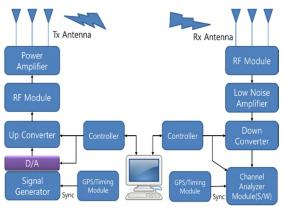
Figure 1. Measurement system configuration
