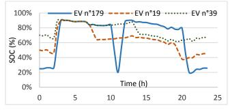
Figure 3. EVs batteries State of Charge (SOC) variation, 2015/02/25
