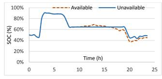
Figure 4. EV n°19 battery State of Charge (SOC) variation 2015/02/25.
