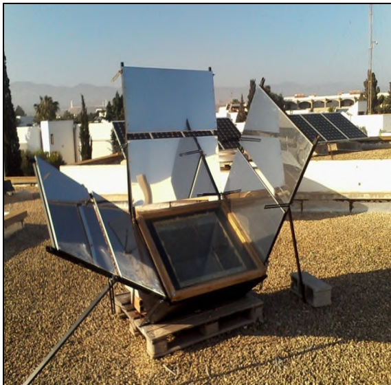
Figure 1. Solar furnace with three external reflectors.
