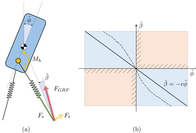
Figure 3. In order for analysis, a new variable  $\tilde{\beta}$  and  $\tilde{\phi}$  are introduced (a). In the domain of variables, the first and the third quadrant are not allowed (b). The controlled relation between  $\tilde{\beta}$  and  $\tilde{\phi}$  must lie within the second and the fourth quadrant.
