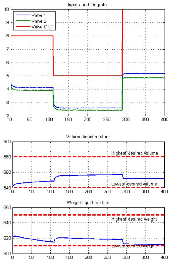
Figure 6. Valver and Results of the DFCM Controller
