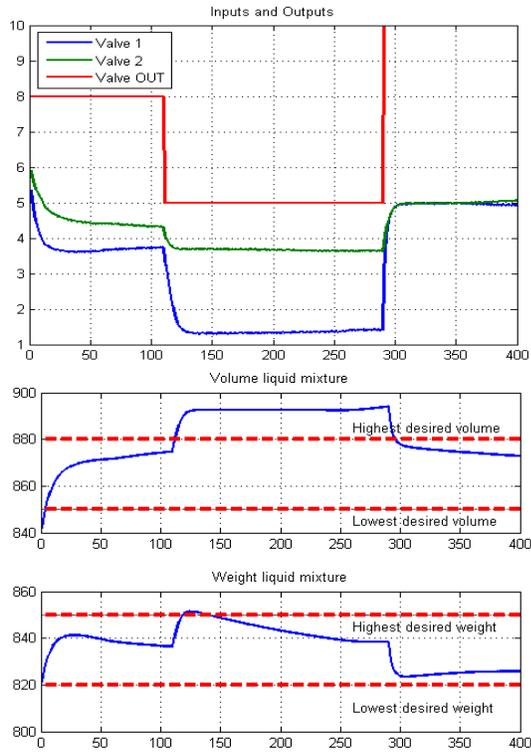
Figure 7. Valves and Results of the Fuzzy Controller
