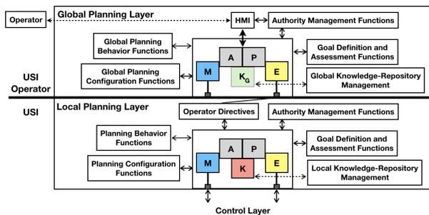
Figure 4. Internal configuration of the Global and Local Planning Layers. The Local (Global) Knowledge Repository is colored red (green) and denoted by  $K$  ( $K_G$ ). Note that  $K$  and  $K_G$  do not necessarily have the same content.
