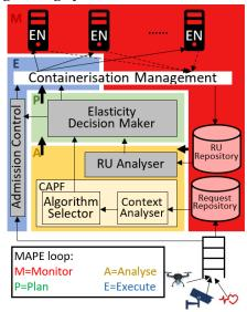
Figure 1. MAPE-based elasticity SAS framework.
