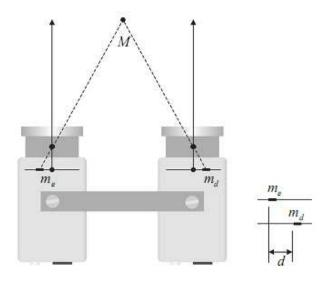
Figure 6. Simplified model of stereoscopic vision([2])
