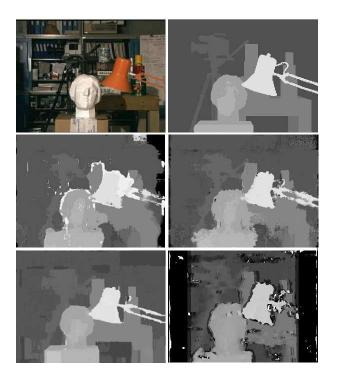
Figure 8. Comparison of disparity maps. a) original image b) expected result; c) result from[13]; d) result from [14]; e) result from [15] f) algorithm from[3] used on this work.
