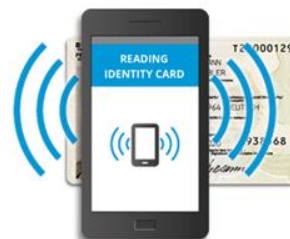
Step (2): The Android smartphone uses NFC to read your private data contactless from your activated eID chip. [Figure 3b]
