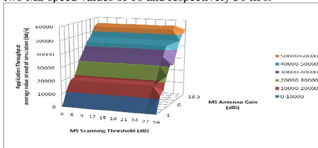
Figure 5. MS Antenna Gain - MS Scanning Threshold -- Decision Space for MS Speed 10m/s
