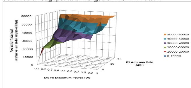
Figure 10. MS Maximum TX Power - BS Antenna Gain -- Decision Space for MS Speed 10m/s
