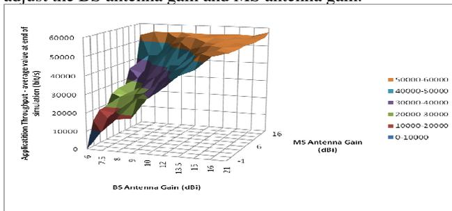
Figure 13. MS Antenna Gain - BS Antenna Gain -- Decision Space for MS Speed 10m/s
