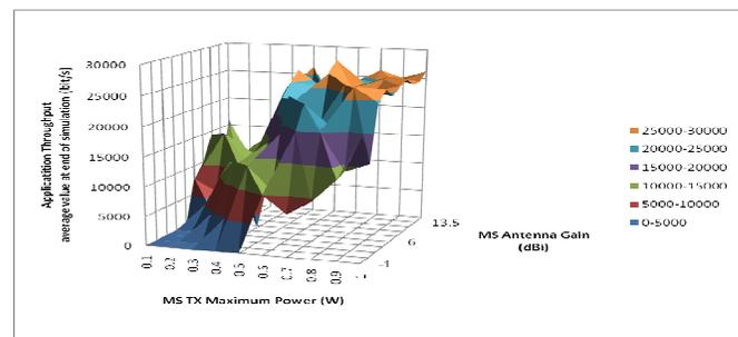
Figure 2. MS TX Maximum Power - MS Antenna Gain -- Decision Space for MS Speed 50m/s
