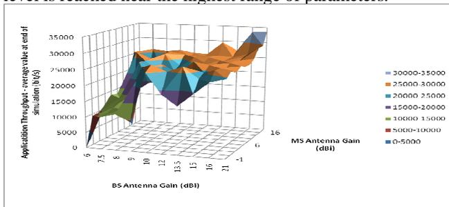
Figure 14. MS Antenna Gain - BS Antenna Gain -- Decision Space for MS Speed 50m/s
