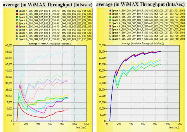
Figure 11. Throughput for different values of MS Maximum TX power and variation of the BS antenna gain (MS TX P = 0.1, 1.0W) s = 10 m/s
