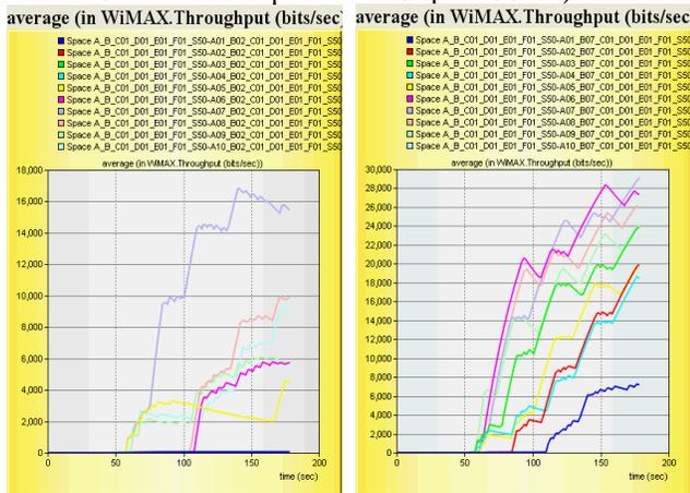
Figure 4. Effect on throughput of Maximum TX power variation conditions, while the antenna gain is fixed ( $g = 0\text{dBi}$  – left, and  $g = 10\text{dBi}$  – right);  $s = 50\text{m/s}$  (180 km/h).
