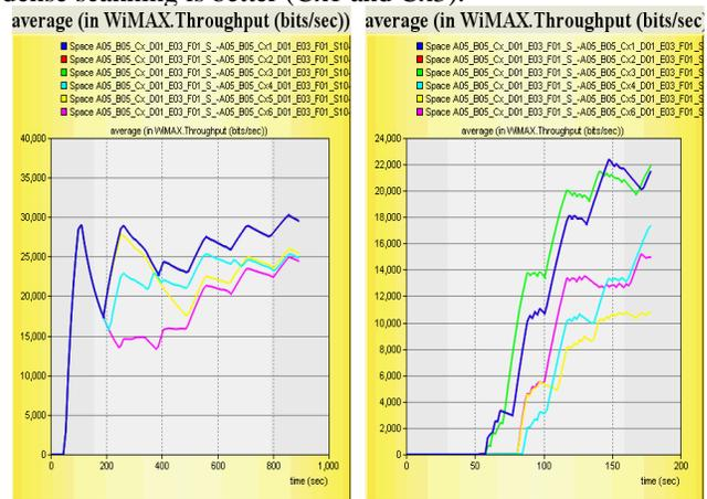
Figure 8. Influence of scanning density, scanning threshold variation and speed on throughput – sample cases
