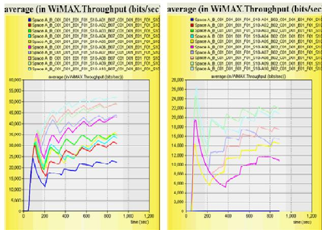
Figure 3. Effect of antenna gain ( $g = 0\text{dBi}$  – left, and  $g = 10\text{dBi}$  – right) on throughput in Maximum TX power variation conditions,  $s = 10\text{m/s}$ .
