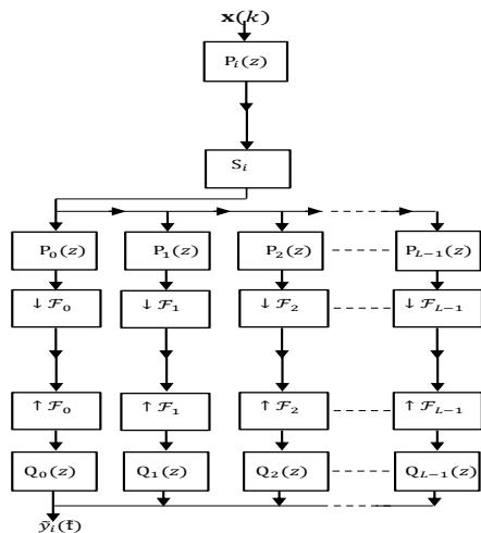
Figure 3.  $i^{th}$  band after implying the maximally sampled filter bank.
