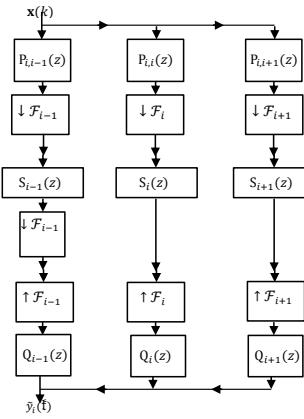
Figure 4. Adaptive filters work at lower rates.
