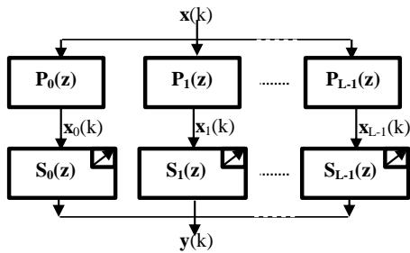
Figure 1. Scheme explains the use of adaptive filters.
