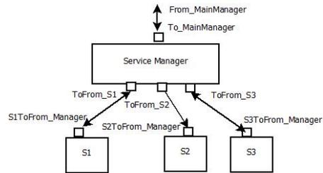
Figure 10. Architecture of triple modular redundancy.
