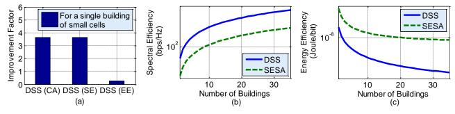
Figure 2. (a) Average capacity, SE, and EE improvement factors of DSS over that of SESA for L=1. (b) SE and (c) EE of DSS and SESA techniques for L>1.
