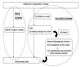
Figure 6. Process introducing the DACS Scheme
