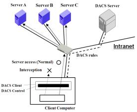
Figure 2. Basic Principle of the DACS Scheme
