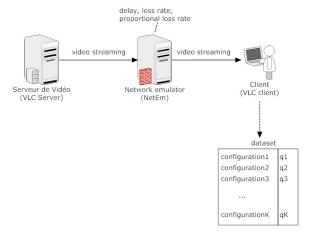
Fig. 6: Testbed for PSQA tool
