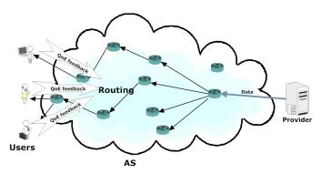
Fig. 1: Integration of QoE measurement in routing system
