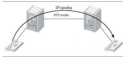
Figure 1. SIP trunking architecture
