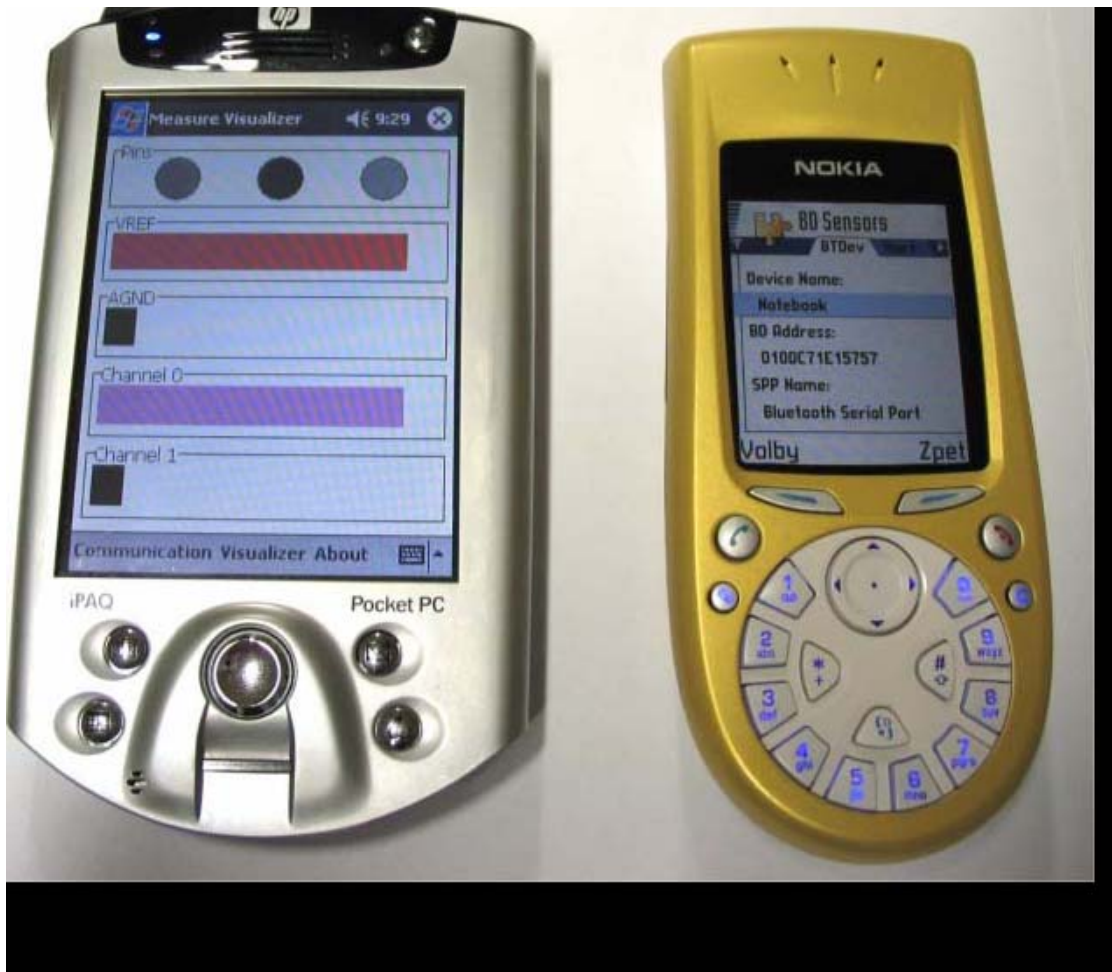
Figure 4. iPAQ PDA 5450 visualizing bar graphs of measured quantities and GSM Nokia 3650 SmartPhone with a sample window for smart sensor parameter settings
