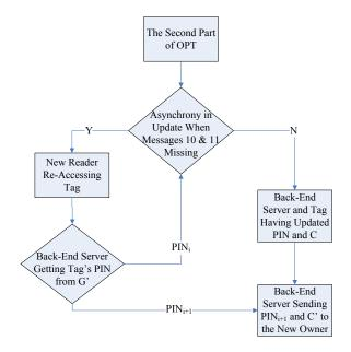
Figure 8. Diagram of OTP When Messages Missing
