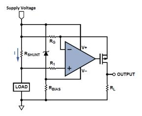
Figure 4. High-current sensing solution using an operational amplifier.
