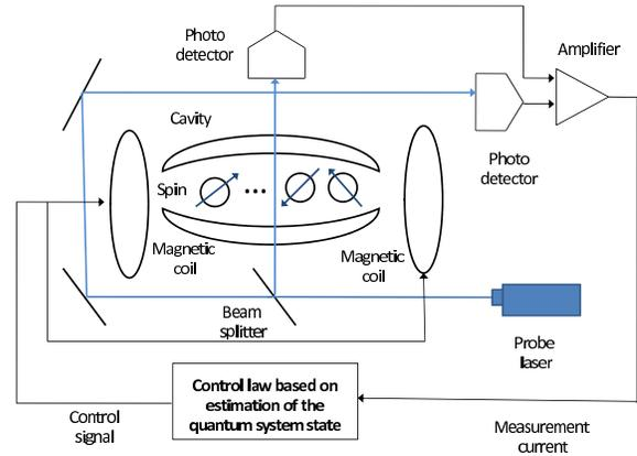
Figure 1. Feedback control loop for quantum systems
