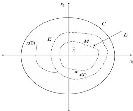
Figure 2. LaSalle's theorem:  $C$ : invariant set,  $E \subset C$ : invariant set which satisfies  $\dot{V}(x) = 0$ ,  $M \subset E$ : invariant set, which satisfies  $\dot{V}(x) = 0$ , and which contains the limit points of  $x(t) \in E$ ,  $L^+$  the set of limit points of  $x(t) \in E$
