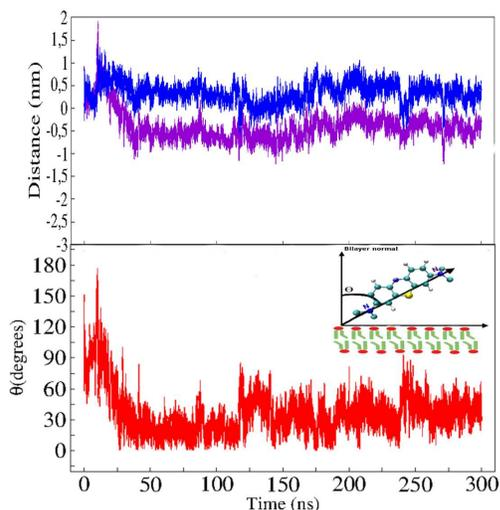
Figure 4. Upper panel: temporal evolution of the positions of the nitrogen atoms with respect to the bilayer/water interface, when ions are considered. Lower panel: temporal evolution of the angle,  $\theta$ , between the nitrogen atoms vector with respect to the membrane-water interface.
